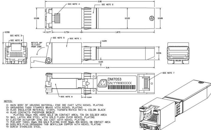
**Figure 2: Mechanical Dimensions**
